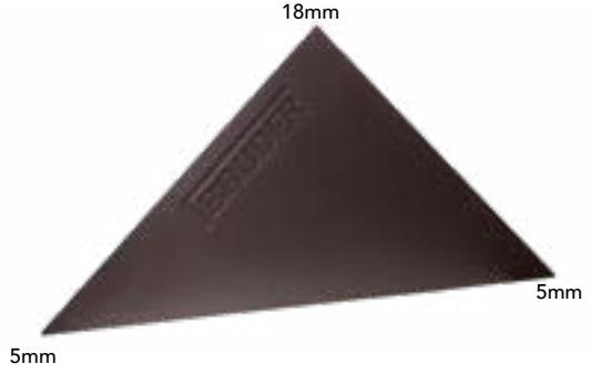
The BauderPIR FA Tapered Insulation is faced on both sides with black aluminium foil to increase thermal efficiency and is available in various thicknesses to achieve the required fall and the desired thermal requirements. The patent-pending unique ridge and valley infill boards are combined in conjunction with the Bauder FA Tapered boards to simplify the scheme and installation.
