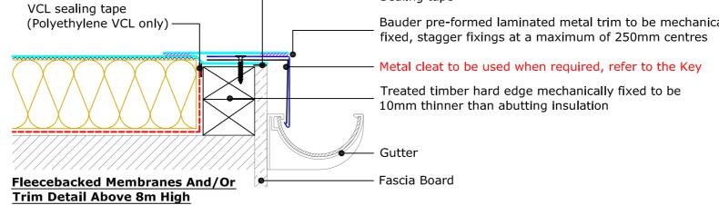
External Gutter - Less than 8m High (Drg.No: D0100-00W\_Ad\_006-005)
