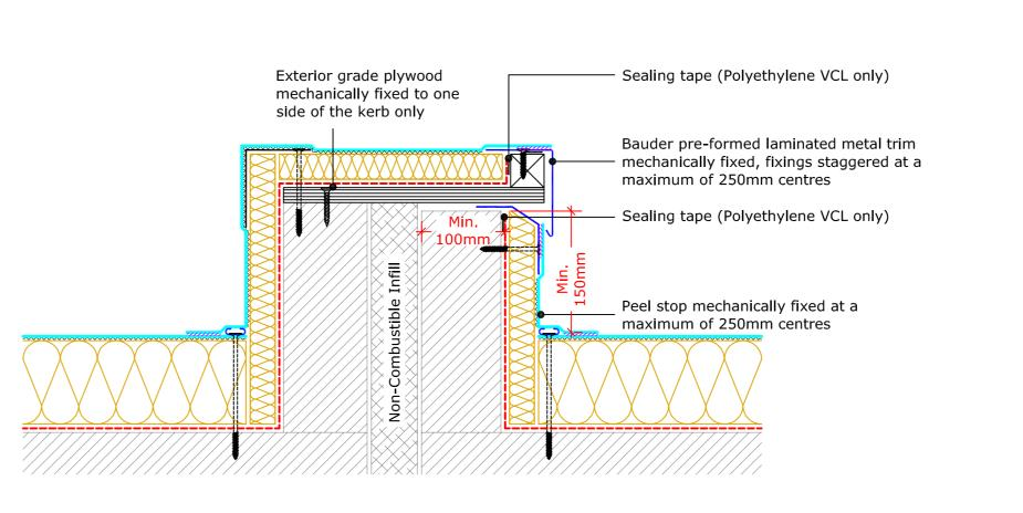
Twin Kerb Expansion Joint (Drg.No: D0100-00W\_Ad\_204-001)
