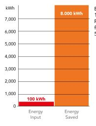
Energy profile for 1m<sup>2</sup> of BauderPIR FA 80mm foilfaced board after 50 year life span
