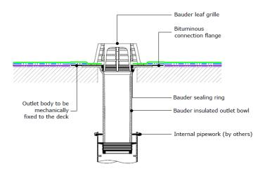
Installation Guidance and data: Please refer to the Bauder Installation Guide and project specification for guidance.
