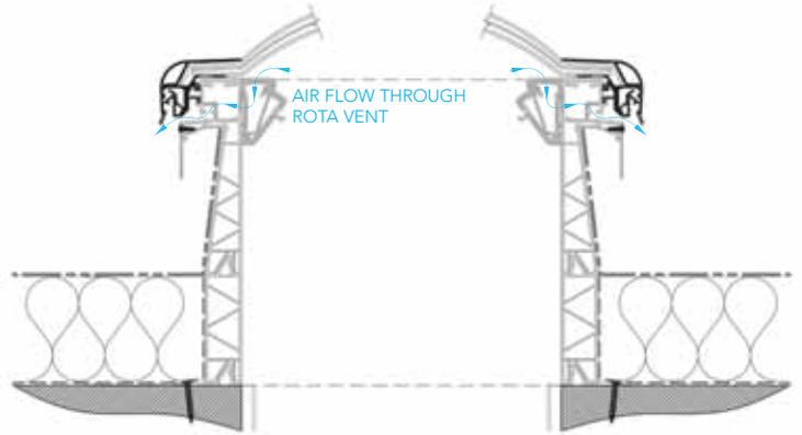
Section through rooflight with rota vent and vertical upstand
