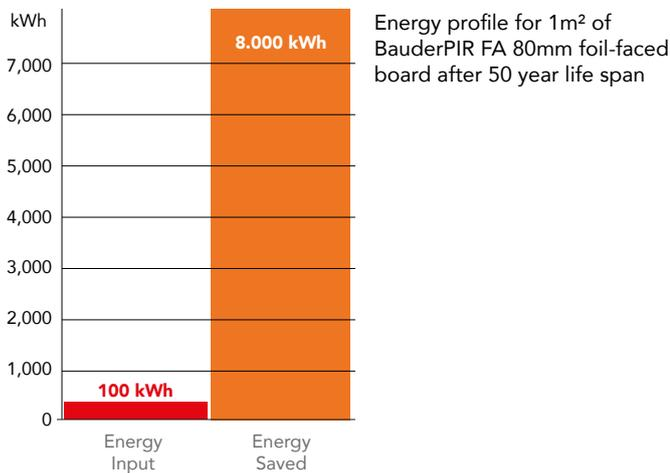
The embodied energy of our rigid polyurethane PIR insulation accounts for as little as 4% of the energy the board can save during its serviceable life. With buildings accounting for 50% of the energy consumption in Europe, the inclusion of insulation when installing new or refurbished roofs plays a significant part in reducing CO<sub>2</sub> emissions.
