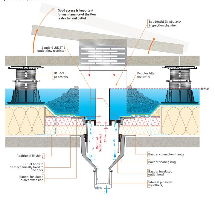
The discharge flow rate is controlled by the adjustable flow Restrictor. The pebble margin filters the rainwater to prevent debris being washed into the restrictor.
