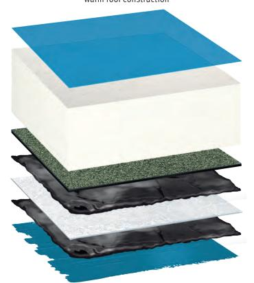
Hot melt waterproofing for inverted roof construction
