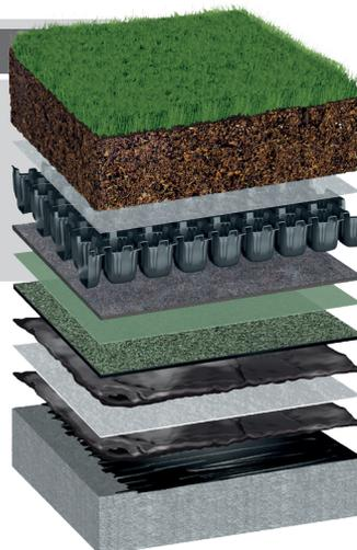
On completion of the waterproofing elements the roof was leak tested to ensure the roof's integrity. The TCRC then installed the Bauder green roof components; PE foil, FSM600 protection membrane, DSE40 drainage layer, filter fleece and over 300 tonnes of Bauder intensive substrate. Finally, Rowland Gold turf was then installed with a drip line irrigation system installed under the turf.
